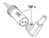
If you use the special Dell plug, align TIP on the Dell plug with TIP marked on the output socket.  $\checkmark$
